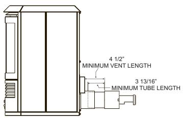
Step 5. Slide co-axial vent pipes into co-axial adaptor. Cut the PVC co-axial pipes at this time. Minimum horizontal vent length 4 1/2" (11.4 cm) Minimum tube length 3 13/16" (9.7 cm)
